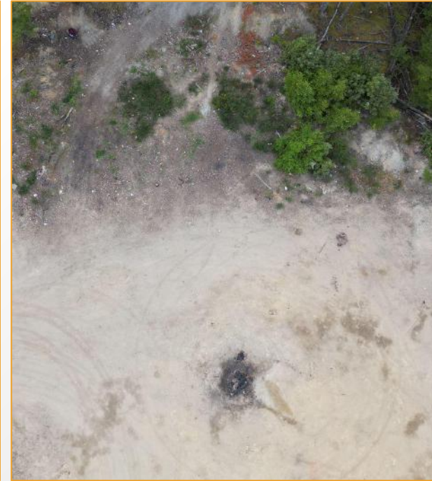
Collapsed potholes in open areas of recreational use
