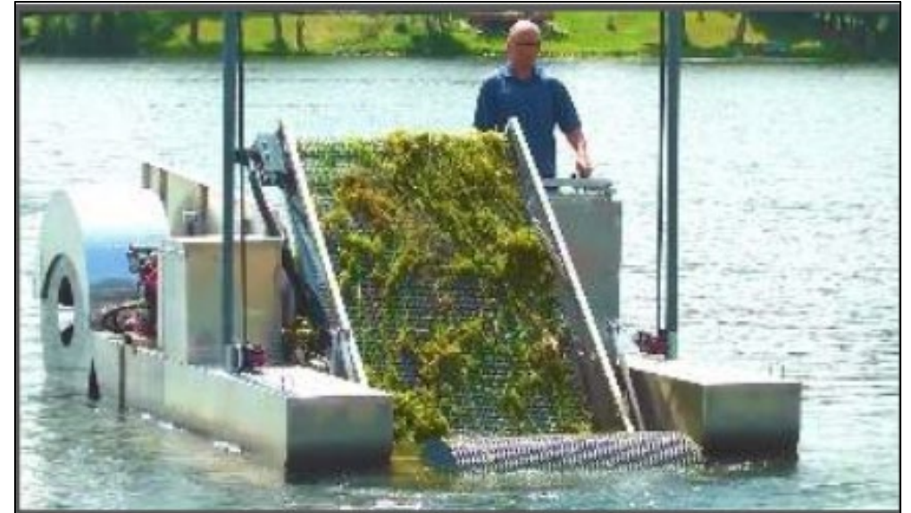
Pulling: Pulls aquatic vegetation instead of cutting, Pulling vs cutting: Reduced floating weed fragments, Can also be used to skim algae: 1.5 acres/hour
