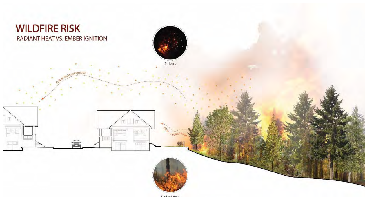
Figure 15 – Radiant heat and ember ignition. During a wildfire, homes are ignited as a result of radiant heat as well as embers carried by wind or convection.
