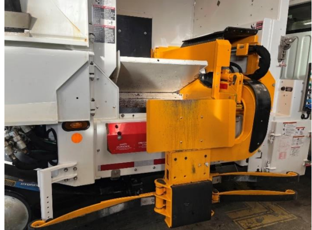
Figure 13: Labrie “Expert Helping Hand” Lift Arm for Cart Tipping
