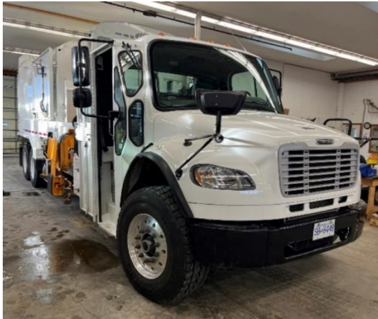
Figure 12: Labrie “Expert Helping Hand” with Stand-Up Cab and Drop Frame Suitable for Manual and Automated Collection
