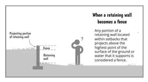
Maximum allowable retaining wall height when combining a retaining wall and fence
