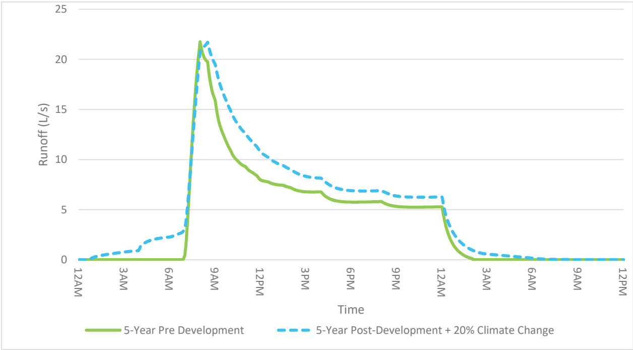
Figure 4: Pre-Development and Post-Development with LID Runoff Hydrographs
