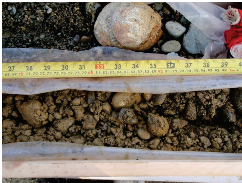
Figure 1: Core drilling in the Boys Road area in March, 2014; photo from well CR-5 from 12-15 m below ground surface (38-48 ft below ground surface) showing the silty gravel and coarse sand layer between the “upper” and “middle” aquifers, believed to be associated with lithology historically described in drill logs as “silty sand and gravel”. The sediments appear to have sufficient permeability to persuade us to combine Aquifer 186 and 187 together as one aquifer. (Photo from S. Barroso, Ministry of Forests, Lands and Natural Resource Operations and Rural Development).
