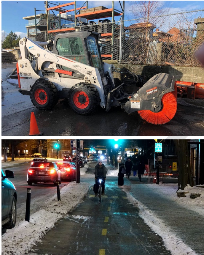
Photo (top) is a Bobcat with rotating brush attachment that the City of Victoria uses to clear snow in its protected bike lanes. Example of a plowed two-way cycling facility in Montreal (bottom). Photo credit: Capital Daily & CBC News
