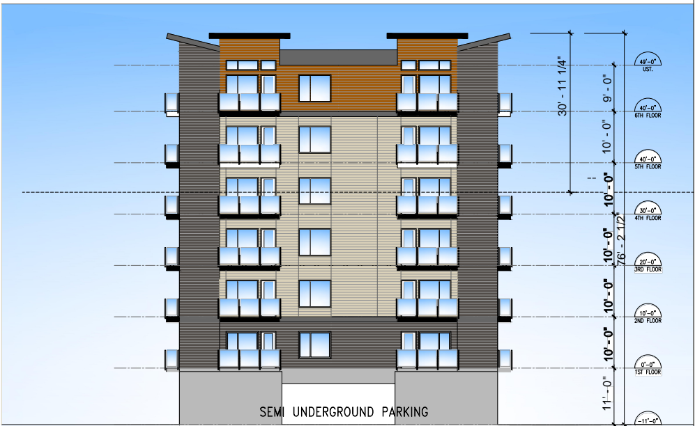
SIDE ELEVATION 6 STOREY ABOVE SEMI UNDERGROUND PARKING
