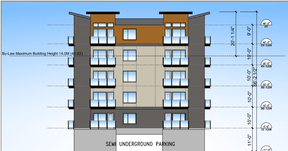
SIDE ELEVATION 5 STOREY ABOVE SEMI UNDERGROUND PARKING
