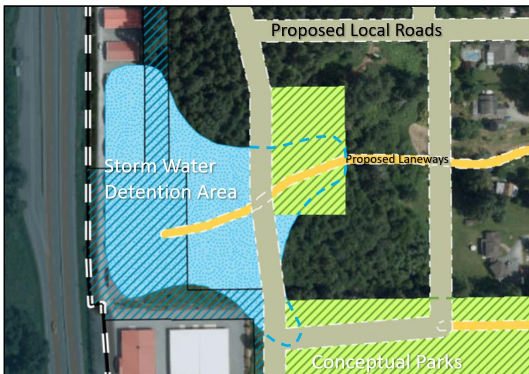
Figure 4: The BMLAP shows local roads running through a storm water detention area and a park. This is an example of a conflict between the proposed transportation network and the proposed Blue-Green Network
