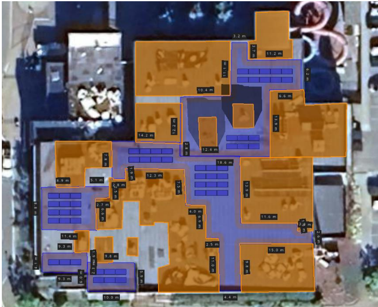
Figure 5-3: Aquatic Centre: Proposed Solar PV System Layout
