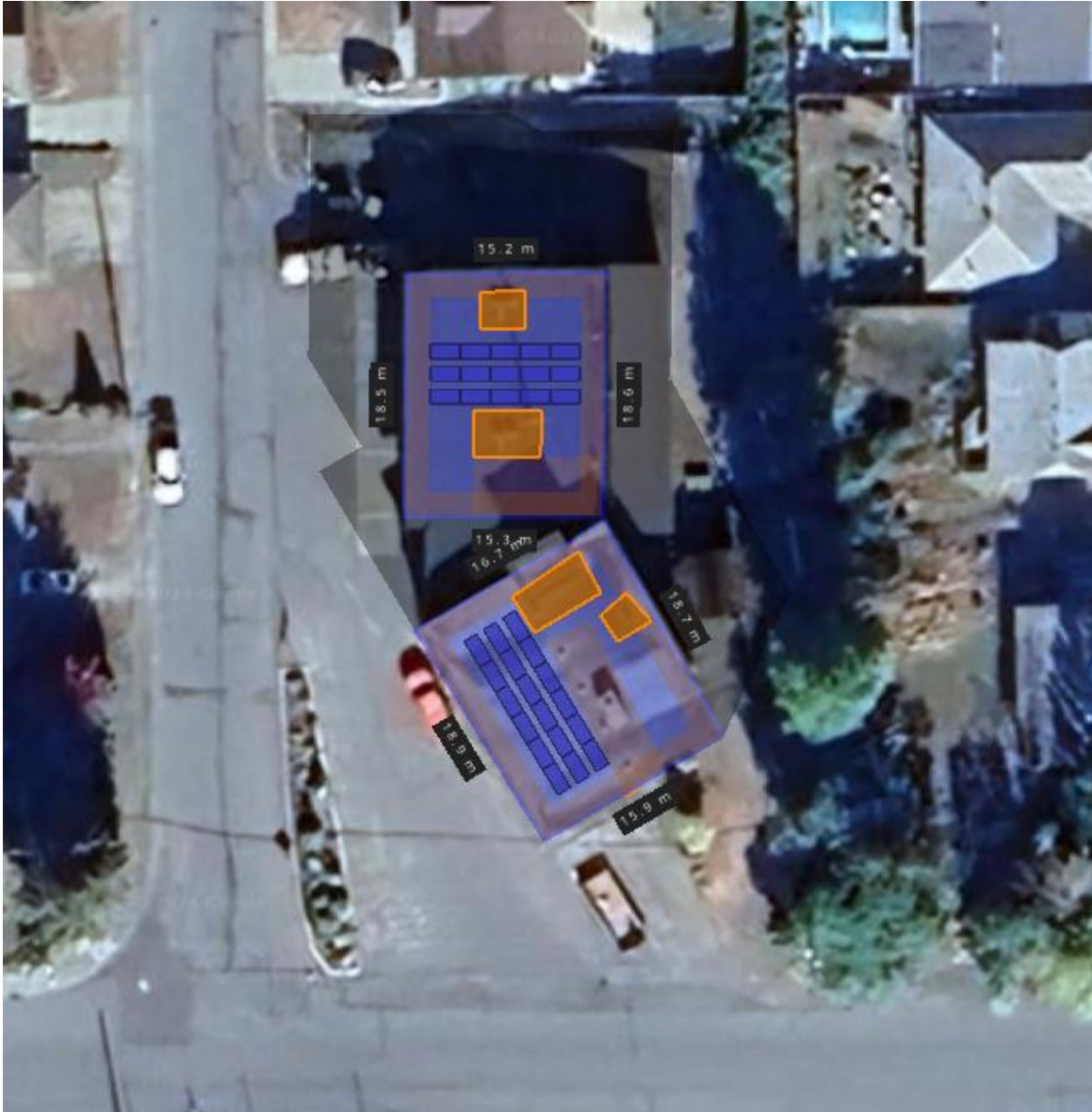
Figure 5-6: Community Firehall: Proposed Solar PV System Layout
