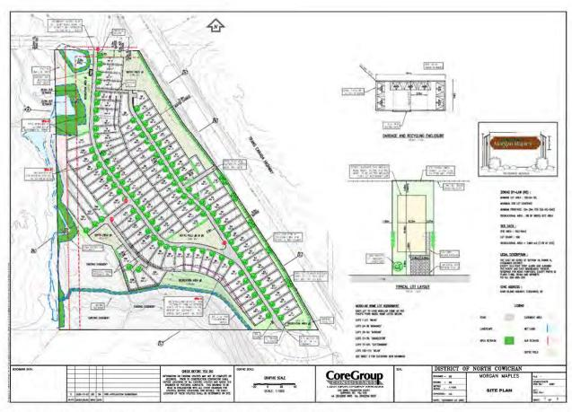
Figure 2. Schematic plan for development. Final unit numbers and lot layouts may vary.
