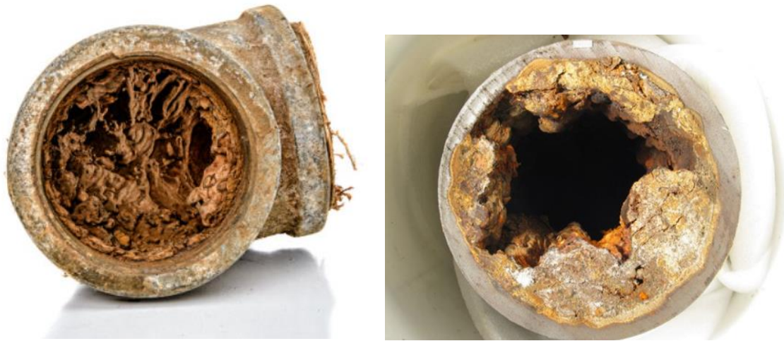
Figure 2 Examples of tuberculated cast iron pipe.
