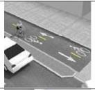
A dashed yellow line should be used to separate two-way bicycle traffic and to help distinguish the cycle track from any adjacent pedestrian area.
